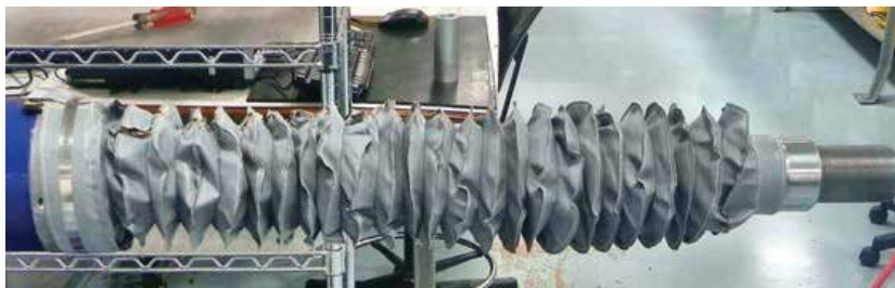
Figure 3: Zippered bellows for ease of installation in the field and adequate protection from the environment
