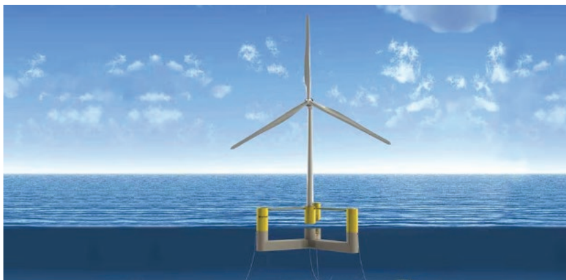
Figure 2: Design of the VoltturnUS [9].
