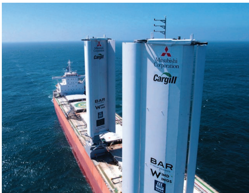
The two WindWings installed on the Pyxis Ocean reduced the energy consumption of the main engine by 32 percent per nautical mile. (Courtesy: © 2024 Cargill, Incorporated)
