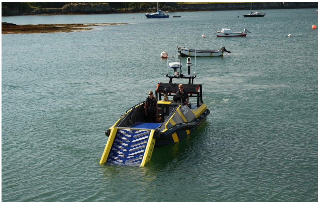
Guardian, an 8.4-meter long, 2.5-meter wide aluminum-hulled Next Generation Fast Rescue Craft, was unveiled to the international maritime industry at the SMM Trade Fair. (Courtesy: Zelim)
