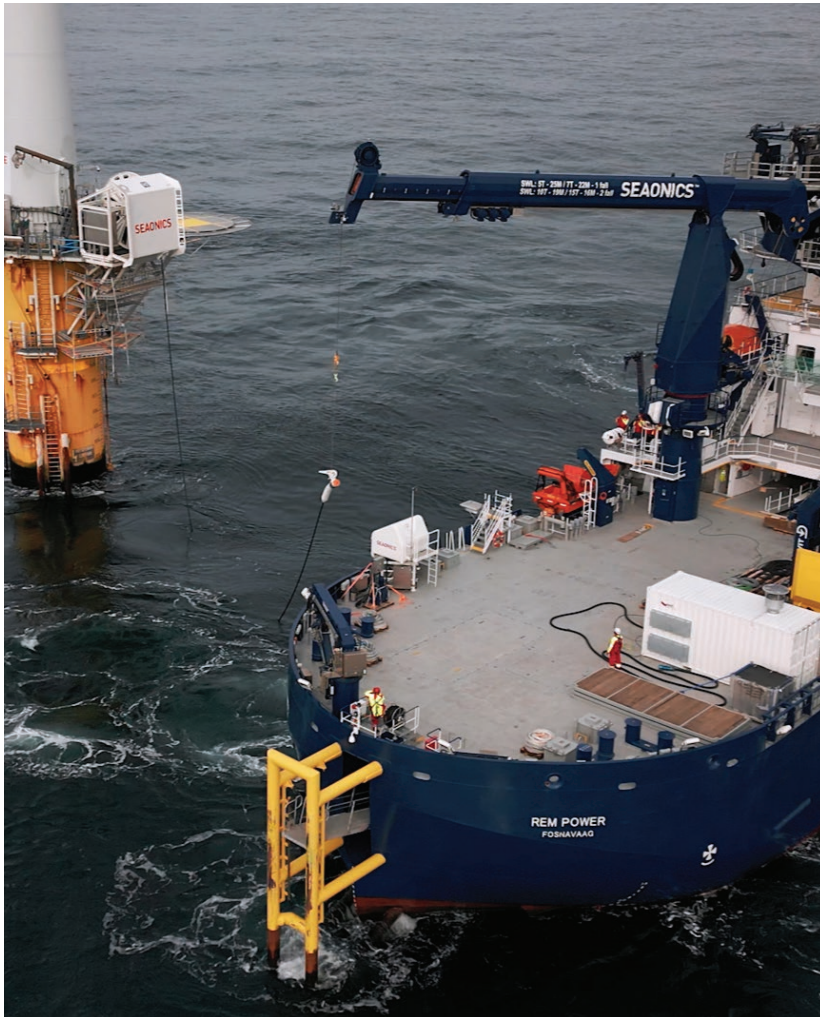
Prototype testing of the Ocean Charger charging the CSOV newbuilding Rem Power from an offshore wind turbine. (Courtesy: Seaonics)
