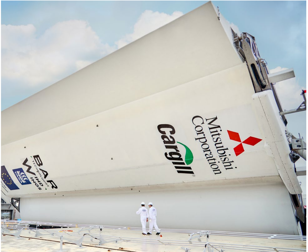
WindWings being retrofitted on Pyxis Ocean at the COSCO shipyard in Shanghai, China, in August 2023. (Courtesy: © 2024 Cargill, Incorporated)
