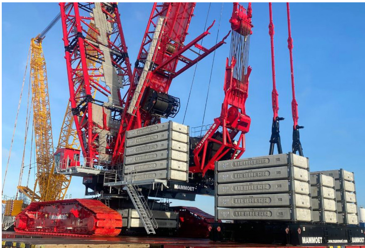
Mammoet's first Liebherr LR12500 crane has a 200m hook height. (Courtesy: Mammoet)
