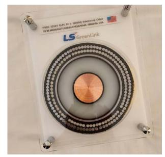
A sample of the HVDC cable that will be manufactured in Chesapeake initially. (Courtesy: LS GreenLink)
