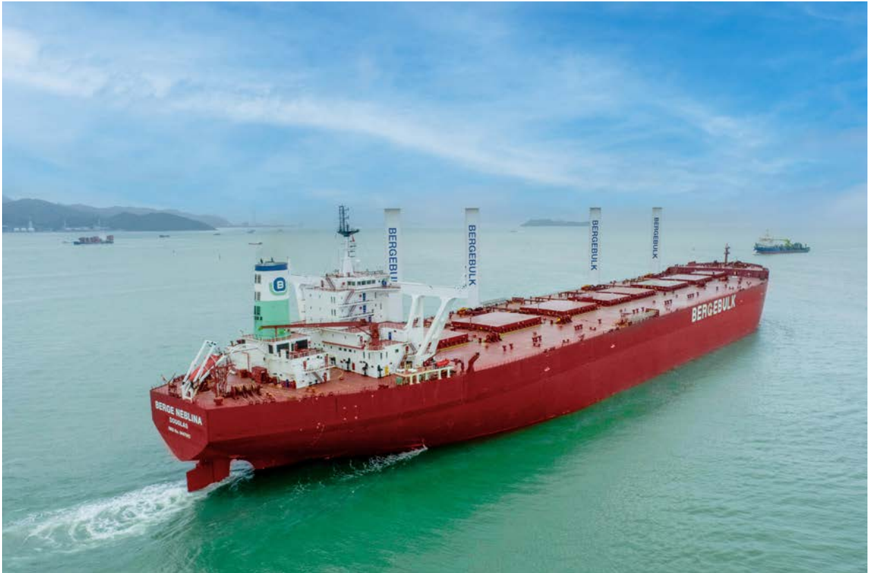
Anemoui's rotor sails harness wind to propel ships. (Courtesy: Anemoui Marine)
