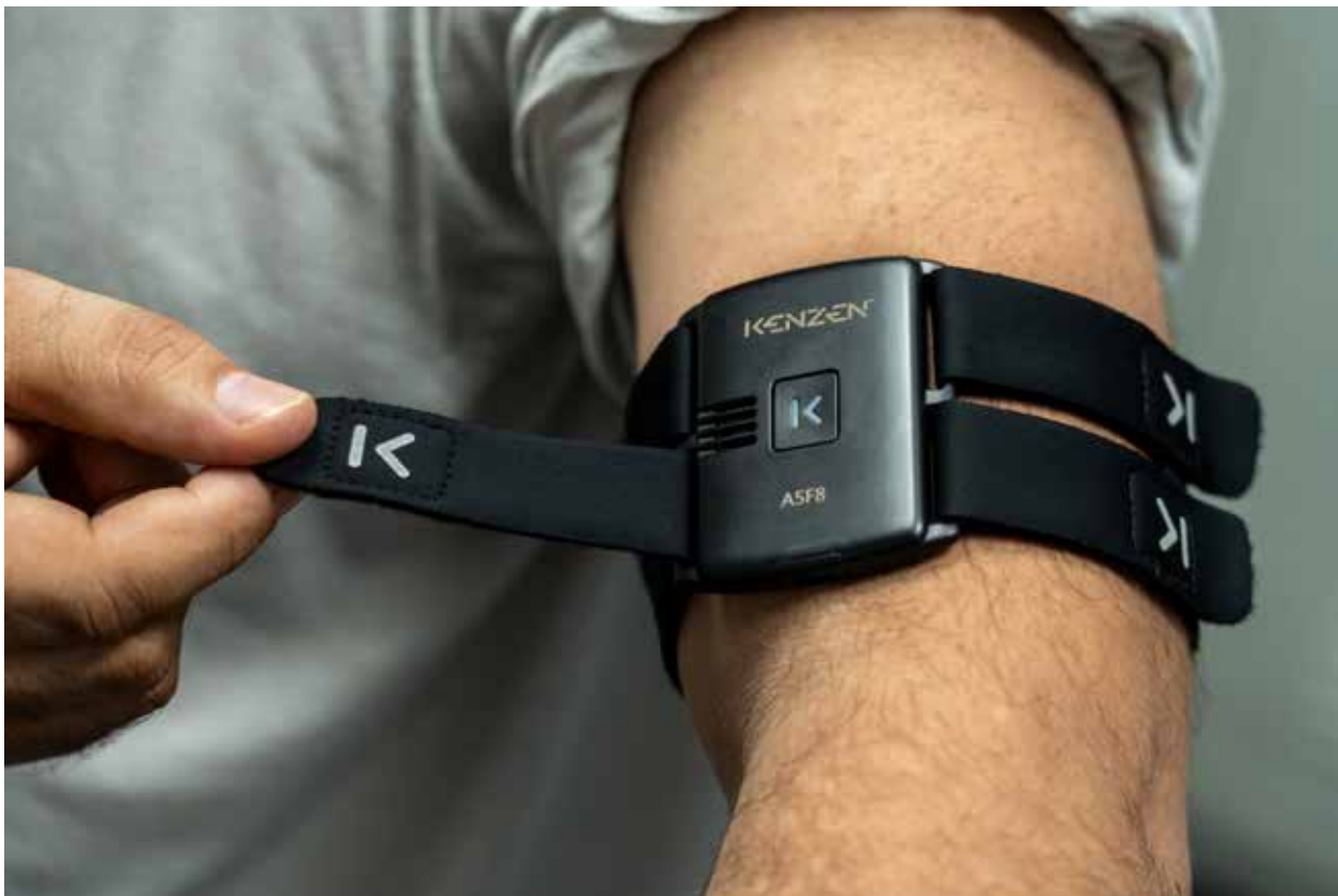
The latest smart PPE innovations include devices worn by workers to monitor physiological indicators such as core body temperature, heart rate, and activity level. (Courtesy: Kenzen)
