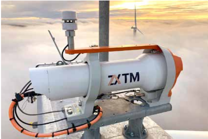
ZX TM is a nacelle-mounted Lidar that uses continuous wave technology to measure the full shear and veer wind profile of a wind turbine. (Courtesy: NRG Systems)
