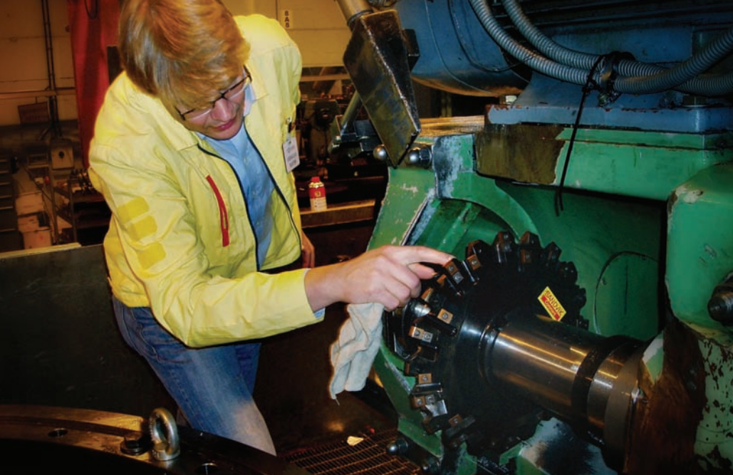
Fig. 1: Milling with a new generation of cutters and indexable inserts are providing higher performance capabilities to gear manufacturing. This indexable insert hob speeds up roughing of gears to higher accuracy levels for finishing.
