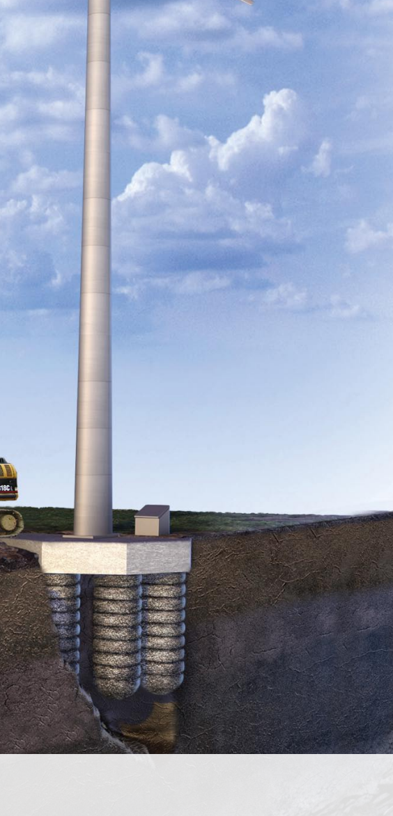
Fig. 1: Rammed Aggregate Pier (RAP) installation.
