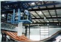
Bridge Crane Impregnator
