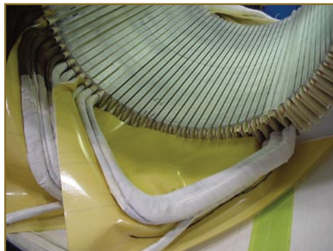
Fig. 2: Upgrading to a class H system allows generators to run at higher temperatures.
