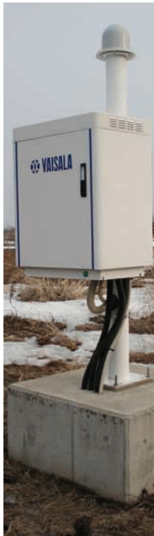
Fig. 3: Vaisala lightning sensor located in Tohoku, Japan, showing mounting pad, mast, electronics enclosure, and antenna assembly.
