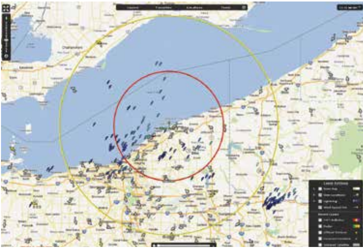
Fig 1: Telvent MxVision WeatherSentry's Wind Edition, showing actual lightning strikes on a map – the rings on the map are wind farms watch and warning ranges.
