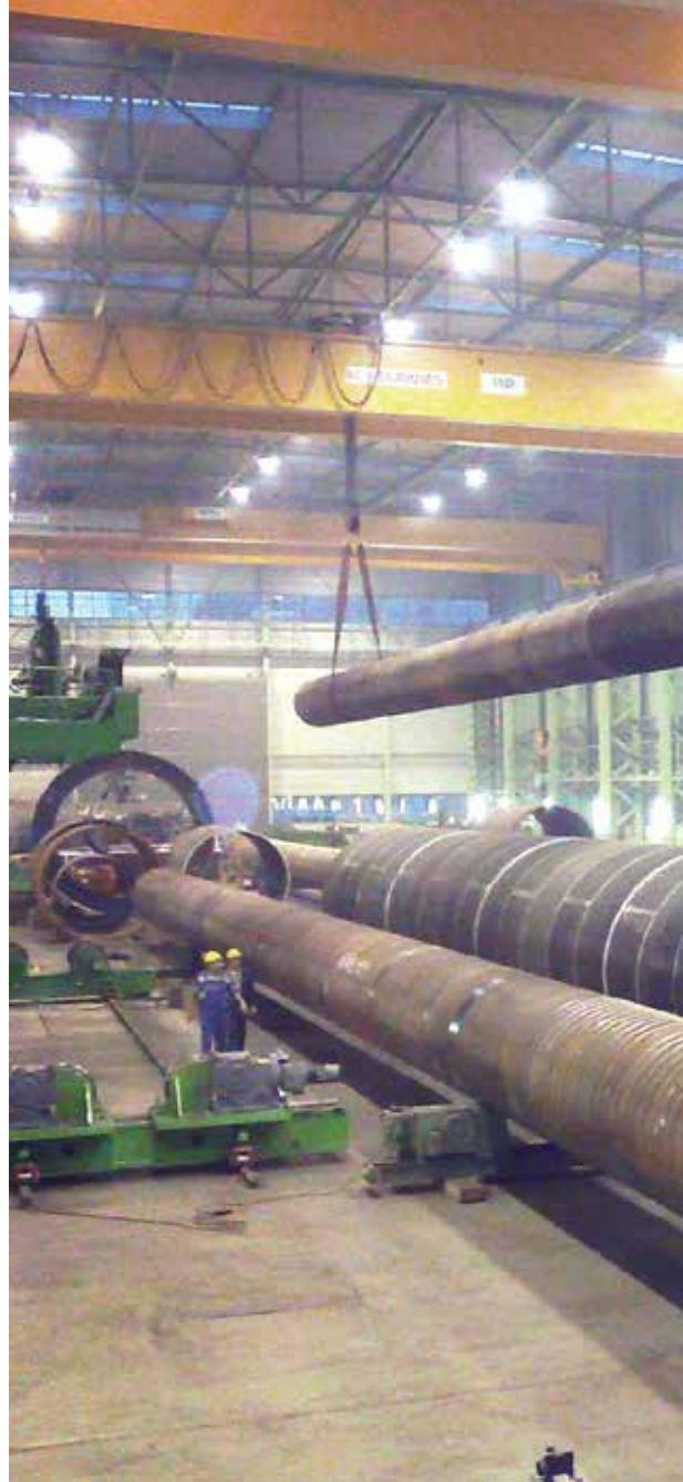
Fig 2: The 60-meter, 400-ton tubes are readied for cutting.
