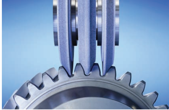
Fig. 1: Maximum OPTI GRIND productivity: An assembly of three dressable wheels rough grinds four tooth flanks simultaneously, as compared to typical use of a single wheel roughing two flanks at once. The center wheel only is then used for finishing, with the desired surface finish and flank modifications dressed into the wheel.
