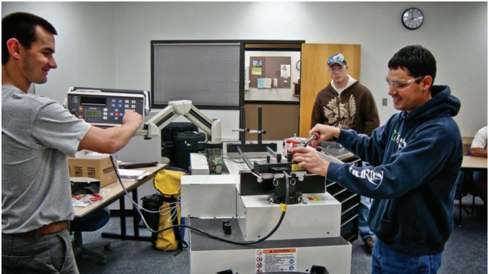
Fig. 3: A student performing torque-tension practice session.
