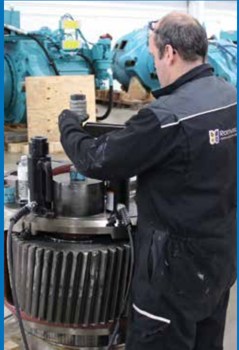
A Romax engineer disassembles planetary stage of a gearbox during failure root cause analysis.
