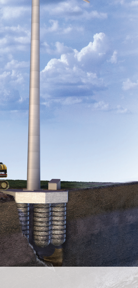
Fig. 1: Rammed Aggregate Pier (RAP) installation.
