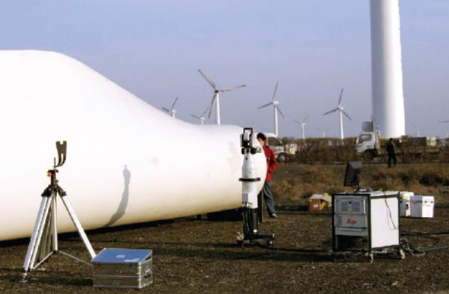
Fig. 3: CMMs can also be set up in the field to check such components as blades.
