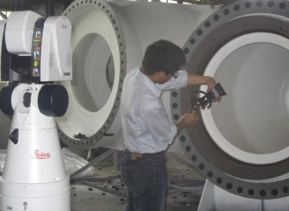
Fig. 2: Inner diameters of a wide variety of components are measured quickly and accurately.
