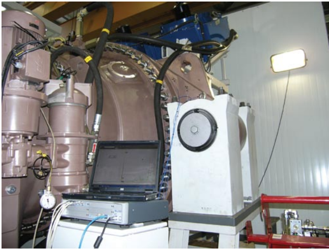
Fig. 5: Visualization is especially helpful to Moventas engineers with the animated mode shapes displayed together on the same screen with plots such as frequency response functions (FRFs).
